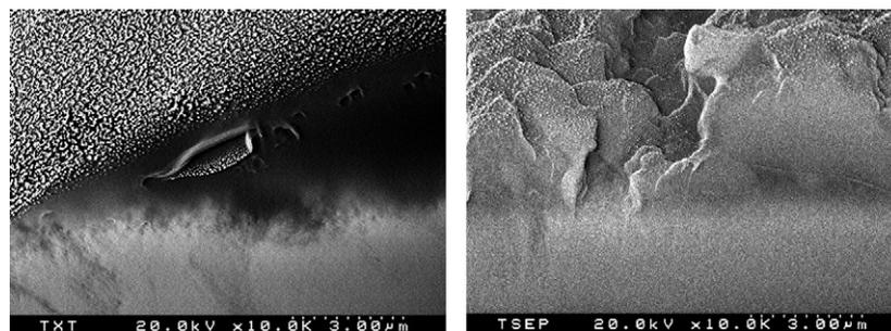
**Fig 3.** Back-scattered micrographs of enamel-adhesives interfaces. Enamel and adhesive are intimately united; contrast offered by back-scattering allows identification of both. **A**, Enamel conditioned with 37% phosphoric acid; **B**, enamel conditioned with SEP (original magnification  $\times 10,000$ ).
