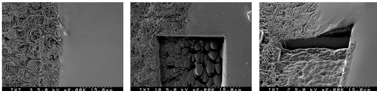
**Fig 1.** SEM images of specimen conditioned with 37% phosphoric acid. **A**, Junction between etched enamel and adhesive before FIB milling. Adhesive surface is smooth, but enamel surface appears etched; **B**, after FIB milling, and **C**, tilted image shows enamel-adhesive interface; penetration of conditioners can be observed (original magnification  $\times 2000$ ).
